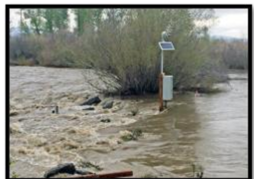
Figure 2. Stream gage during flooding event.
